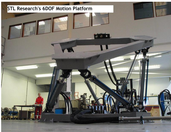
Figure 2: Six degree of motion simulator in use at the STL Research facility
