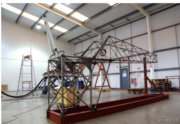
Figure 4: Lightweight steel-truss arm sections for validation of stress and deflection predictions
